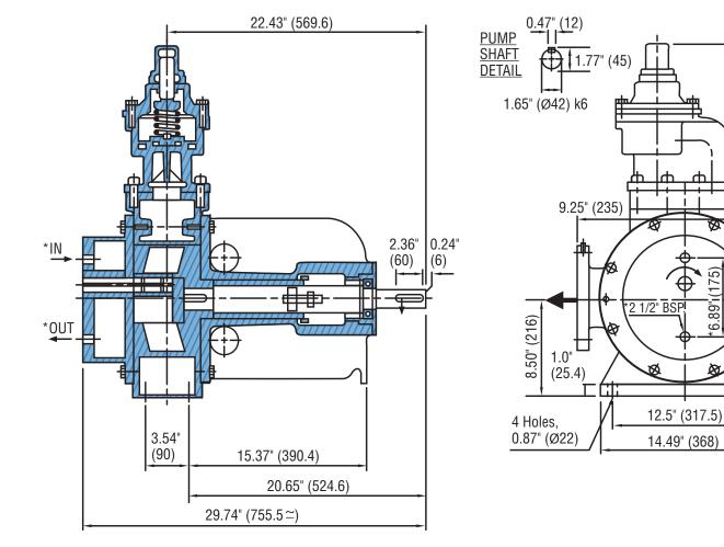
DIMENSIONS IN INCHES. ALSO SHOWN (mm). \*OPTIONAL HEATING JACKET SHOWN WITH (2)1/2" THREADED CONNECTIONS.
